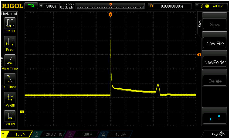
Plead signal at 800 RPM & 14.2 volts (zoomed in)
